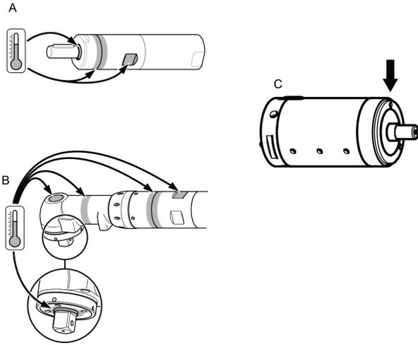
The highest temperatures occur when the motor is running at full pressure without load. With increasing torque, the air motor reduces the rotational speed and the temperature.
